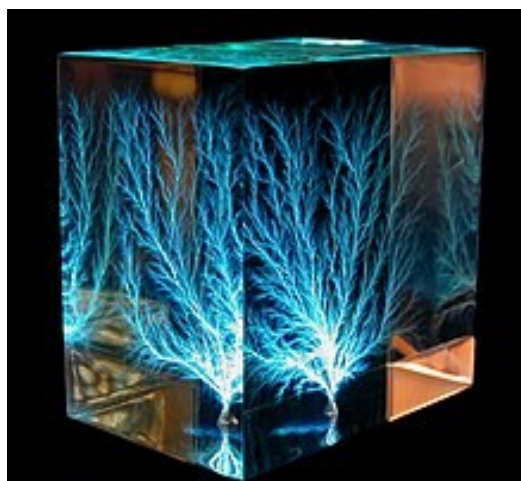
Figure 2.35: A Lichtenberg figure
